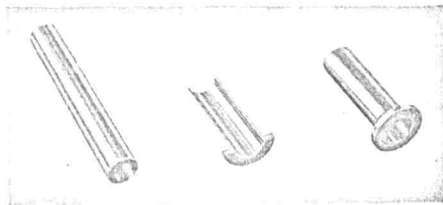
Fig. 14. Tubing flanged under high pressure.
